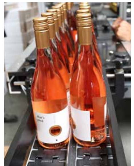
The wine bottles are transported to the packing station on a conveyor section.
