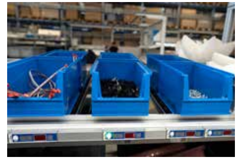
Worker guidance by pick-to-light: Light signals indicate from which box the next material is to be taken.
