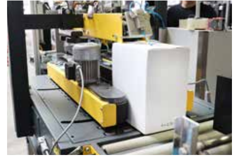
After packing the cartons are sent for automated labelling.
