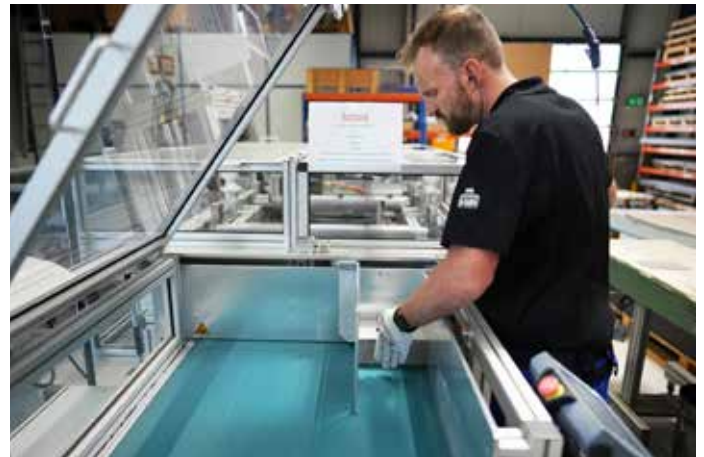
On inserting the components, a stop ensures their precise orientation.
