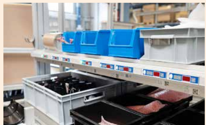
The material is supplied from the back by kanban.
