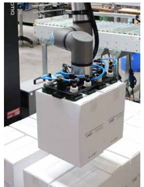
A robot places the wine boxes on pallets.
