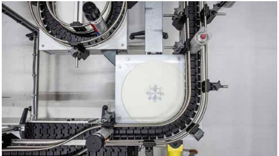
MiniTec segmented chain conveyors allow different curve radii.
