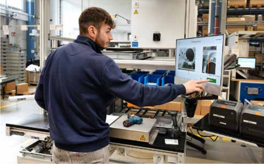
The assistance system provides step-by-step guidance through the assembly process.
